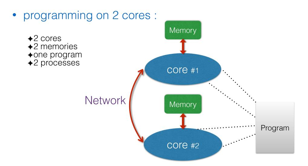
Sketch of a two cores calculation
